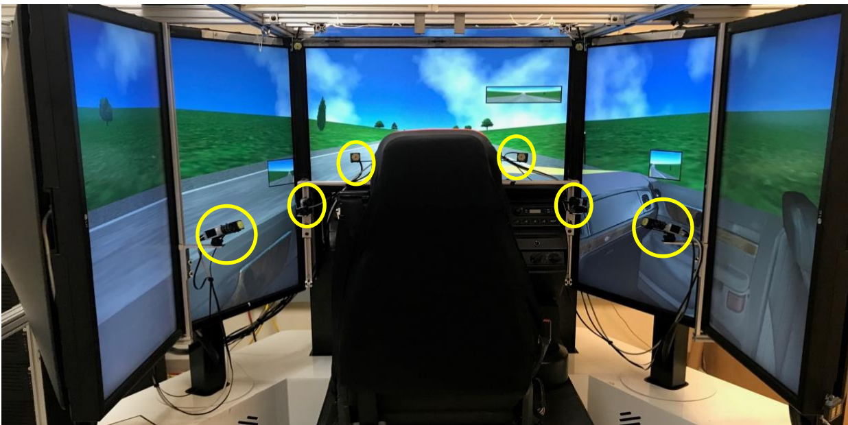
Figure 1. FAAC® driving simulator with SmartEye® 6-camera head and eye tracking system (yellow circles).
